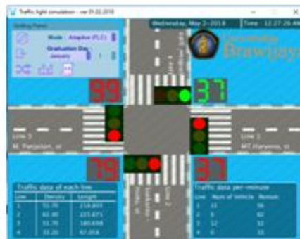
Figure 2 The Traffic Lights Controller Simulations
